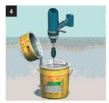
Mix Sikadur®-31 C components A and B for a minimum of 3 minutes until the mix is homogeneous.
