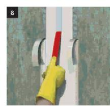
Remove the red middle strip and the masking strips on both sides to ensure a neat and precise detail.
