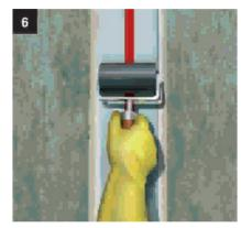
Press the Sikadur-Combiflex® SG tape without trapping air into the adhesive by using a suitable roller. The adhesive should be squeezed out on both sides by ~ 5 mm.
